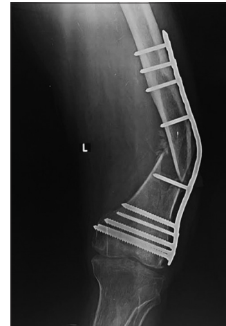
Figure 9: Anterior posterior radiograph of the femur showing a bent plate. During the initial phase of mobilization, the plates bear the load. Once the fracture gets “sticky” the bone starts to “share” the load. In the absence of a callus, the entire weight is taken by the plate, as seen in this case, leading to eventual failure.
