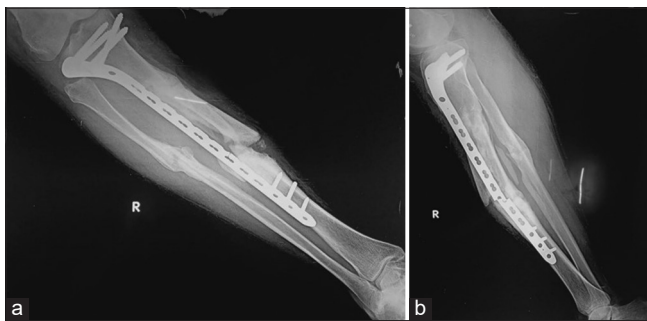
Figure 2: (a) Anterior posterior (AP) and (b) lateral radiograph of the leg showing buttress plate with fixation screws proximally for fracture mid shaft of the tibia, showing atrophic non-union, due to rigid fixation and distraction at the fracture site. Also note implant failure was identified clearly on lateral view only, seen as a faint fracture only on the AP view. It is seen at the screw hole, which is the weakest point in a plate. The soft-tissue density with linear opacity identified on the lateral view is artefactual.
